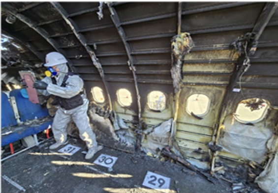
Location of overhead bin where fire occurred
