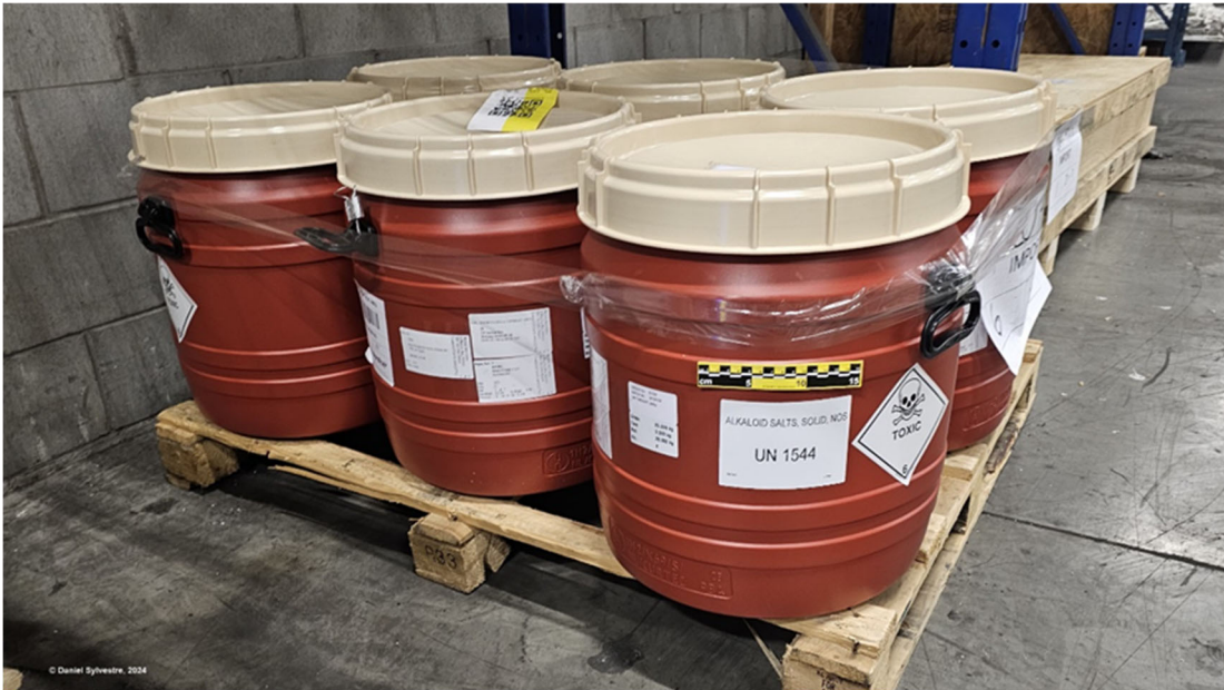
Figure 1. Consignment of UN 1544 alkaloid salts, solid, n.o.s. (note the absence of a technical name)
