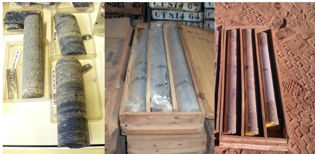
Geologic carrots (rocks, 8 cm in diameter, up to 1 m long, up to 15 kg each) in plastic tubes closed by adhesive tape, or in plastic sleeves, placed in a rack, made of plywood or natural wood
