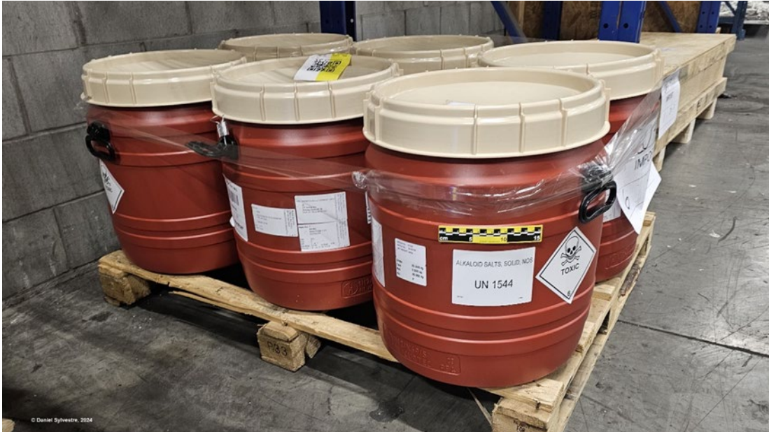
Figure 1. Consignment of UN 1544 alkaloid salts, solid, n.o.s. (note the absence of a technical name)
