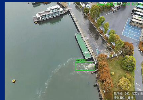
Sewage Outlet Identification
