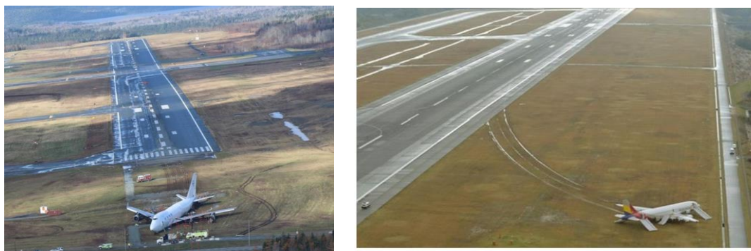
Figure 6: Aeroplane overshoot and veered off from runway
