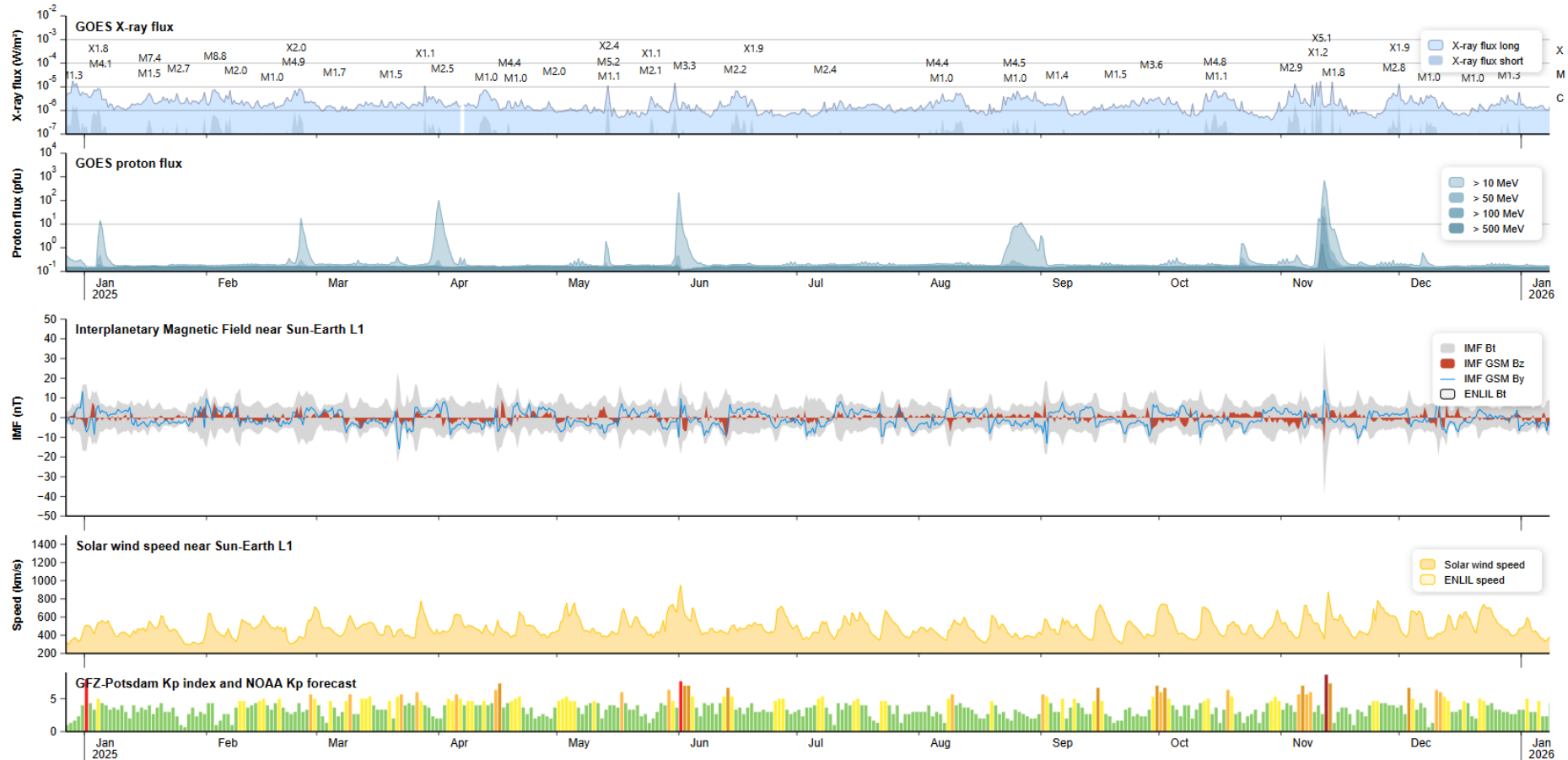
Figure 3. Overview of the solar and geomagnetic activity in 2025. The figure shows from top to bottom: solar X-ray flux (flaring activity), solar proton flux, interplanetary magnetic field, solar wind speed, and K_p index. Solar X-ray flux and solar proton flux are measured near the Earth by the Geostationary Operational Environmental Satellites (GOES) (source NOAA SWPC). Interplanetary magnetic field and solar wind parameters are measured by the Advanced Composition Explorer (ACE) and Deep Space Climate Observatory (DSCOVR) satellites (source NOAA SWPC). The bottom panel shows the geomagnetic activity indicator K_p (source GFZ Potsdam).
