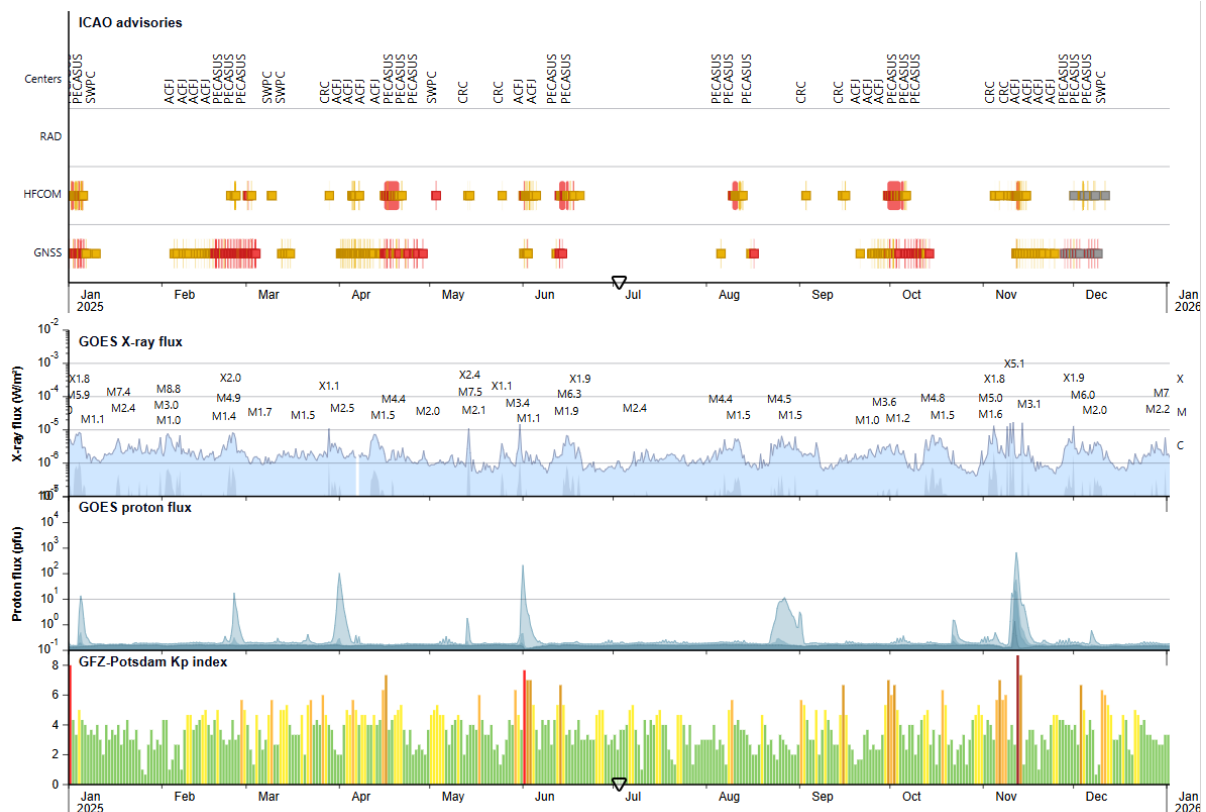
Figure 1. An overlay of when the advisories were issued by each of the SWXCs compared to solar and geomagnetic activity in 2025. The top panel indicates which centres were on duty when RAD, HF COM, and GNSS advisories were issued. Shaded squares and lines show the individual space weather events with yellow representing MOD and red representing SEV. The second and third panels show the X-ray flare activity and relativistic proton flux which are measured near the Earth by the GOES satellite. The bottom panel shows geomagnetic activity indicator Kp (source GFZ Potsdam).
