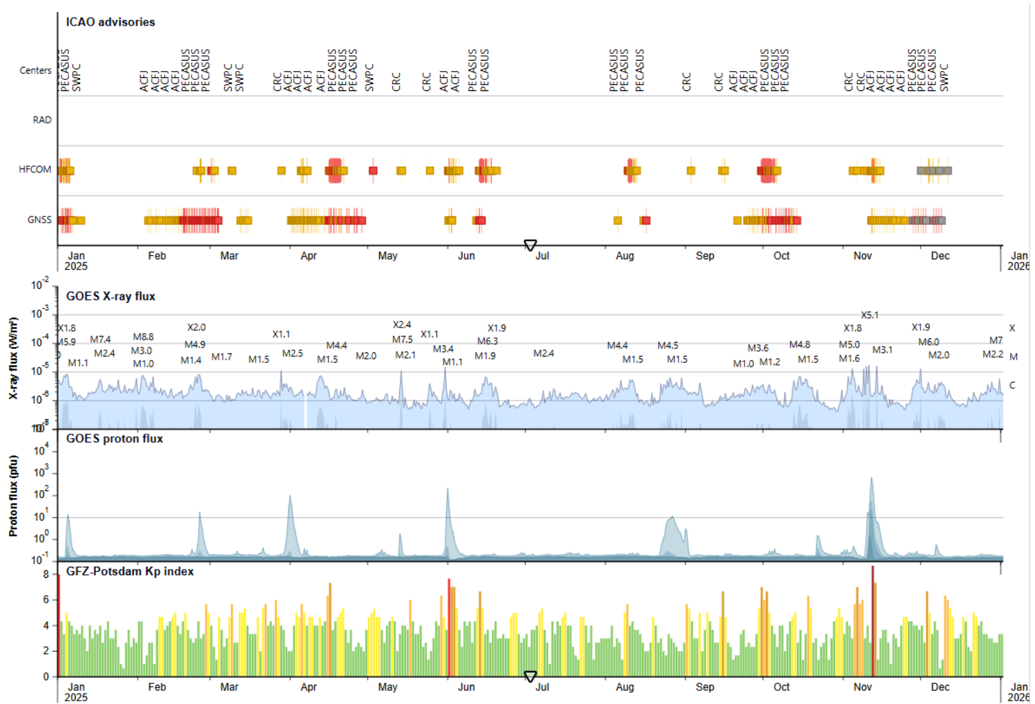
Figure 5. An overlay of when the advisories were issued by each of the SWXCs compared to solar and geomagnetic activity in 2025. The top panel indicates which centres were on duty when RAD, HF COM, and GNSS advisories were issued. Shaded squares and lines show the individual space weather events with yellow representing MOD and red representing
