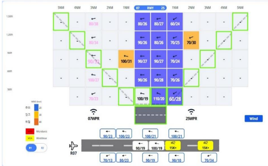
Figure 2. Textual and numerical display of wind and wind shear information at Jeju International Airport
