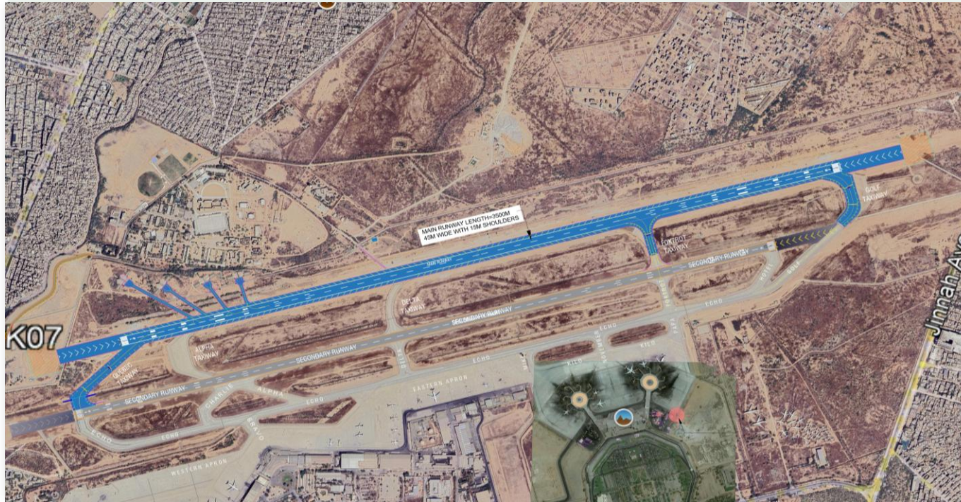
Karachi (JIAP) — two-runway configuration. 07L/25R reconstructed and extended; operations sustained on 07R/25L.
