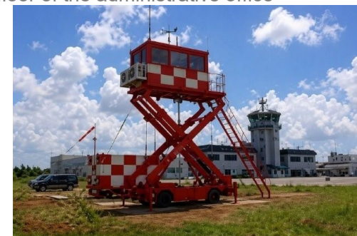
Deployed EVA Maximum wind gust during deployment : 25m/s
