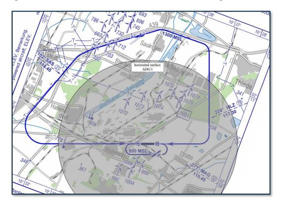
The horizontal surface is not protecting the visual circuit pattern in this instance
