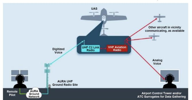
This infographic details the various aspects of Aura's commercial network, which is designed to enable remotely piloted flight operations in controlled airspace. © Aura Network Systems
