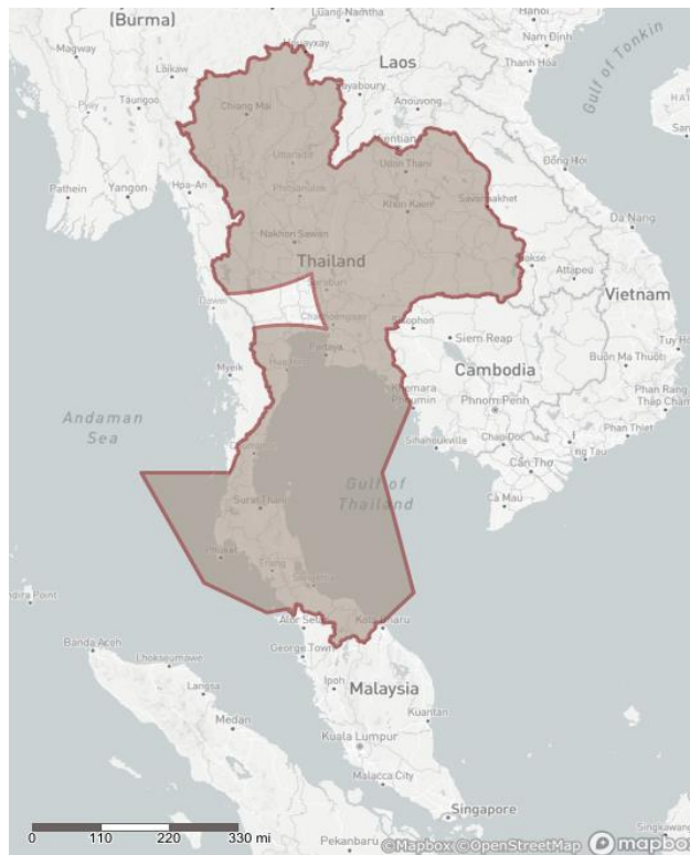
Figure 5 – Intersected coverage of SSR, ADS-B and Bangkok FIR
