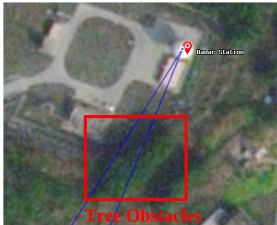
Target missing and erratic track caused by Trees occlusion
