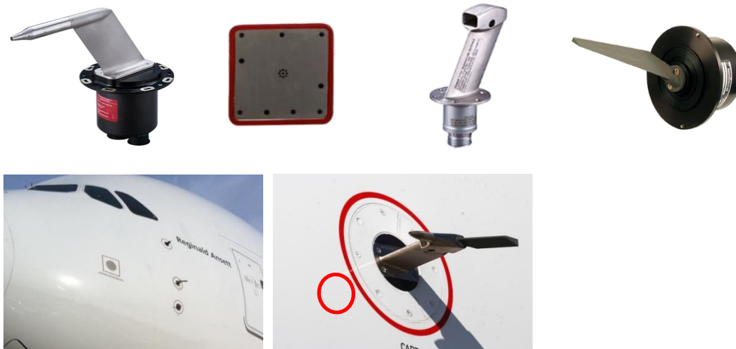
Figure 3.7 Air Data Sensors and Integrated Sensor on Airbus A380
