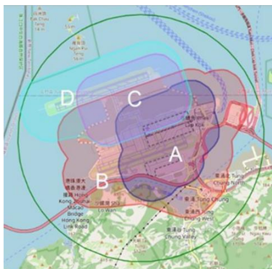
Figure 1 The designated lightning alerting zones ‘A’ - ‘D’ over the HKIA.
