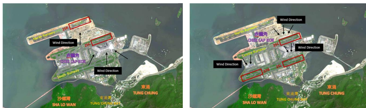
Figure 2. Possibility of building-induced low-level wind effects on landing and departure at HKIA
