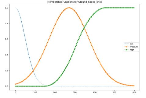
Cruising is characterized by high ground speed, high altitude, and low rate of climb.
