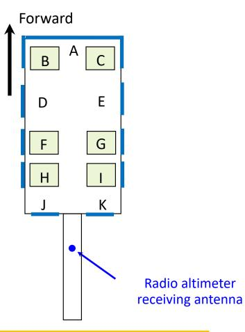
The minimum IPL values is 49.2 dB, obtained at line-of-sight condition with the RA antenna.
