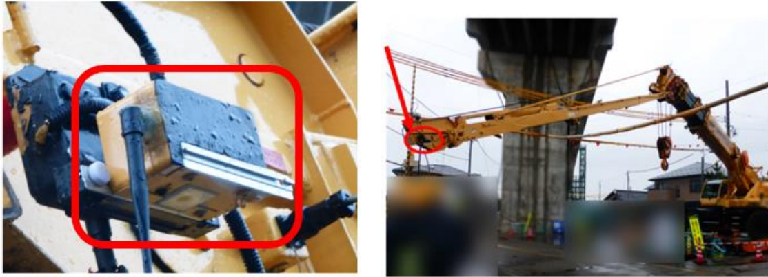
Figure - 3 The RFI was caused by a wireless camera mounted on a crane at a construction site.
