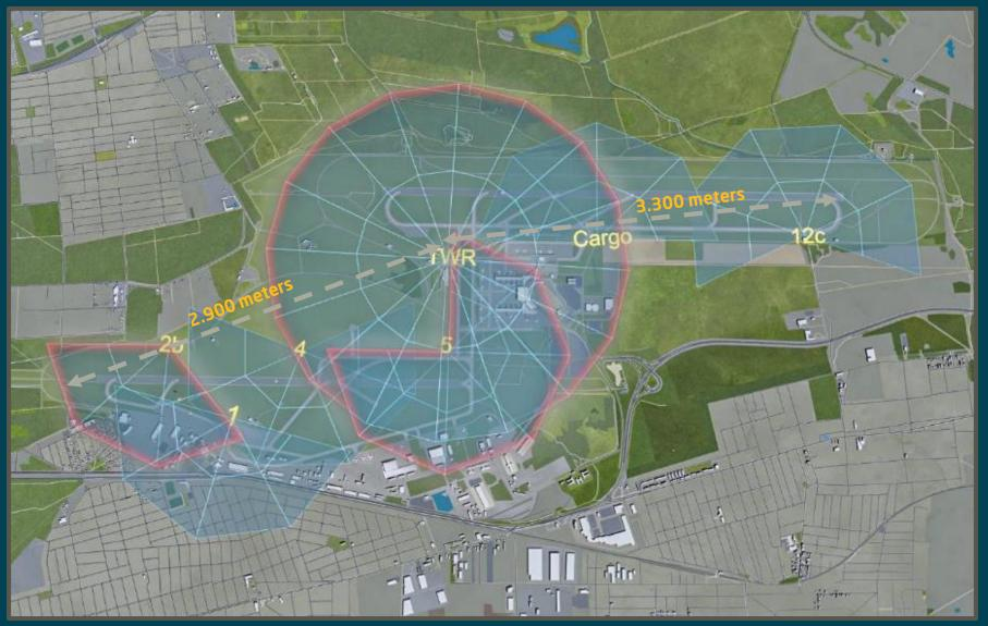
Multi-mast digital tower visual system (1 mast with 360° view + 6 additional masts) for a perfect visual coverage of the airport
