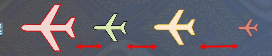
80s average separation means 40 landings per hour86s average separation means 42 landings per hour
