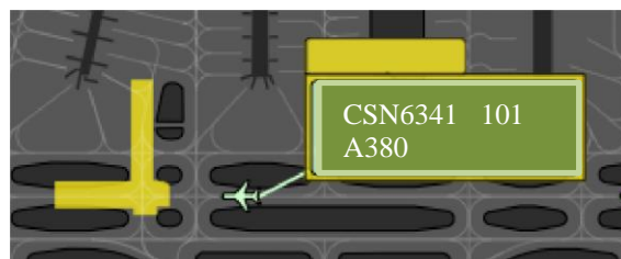
Figure 3An Alert Triggered When An Aircraft Nears the Construction Area.
