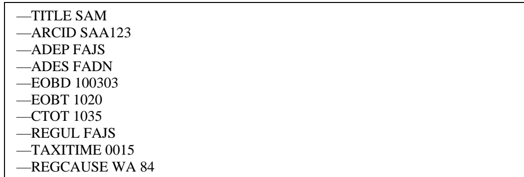
Figure 5: SAM message using ADEXP structure
