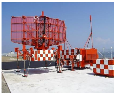
Figure. 2 and 3 Emergency radar facility (antenna and control room)
