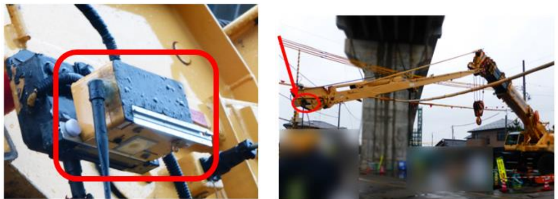
Figure 3. The RFI was caused by a wireless camera mounted on a crane at a construction site
