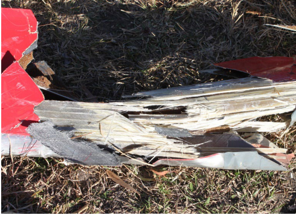
Carbon fibre in aircraft skin
