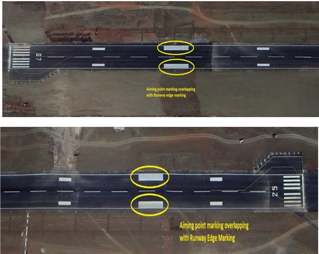
Figure 4: Overlapping of Aiming Point Marking and Runway Side Stripe Marking
