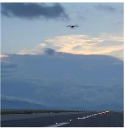
(b) Drone to perform orbiting to measure DVOR bearing error
