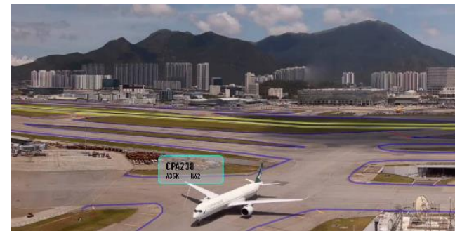
Detection and labelling of an aircraft on taxiway
