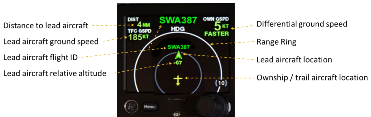
Figure 1 – ACSS avionics being installed in AAL A321s (the only new hardware is the AGD) Copyright ACSS. Used by permission.
