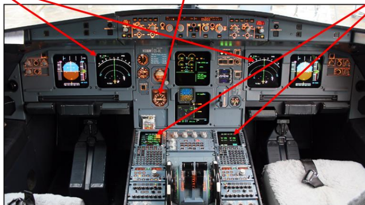
Figure 1 – ACSS avionics being installed in AAL A321s (the only new hardware is the AGD) Copyright ACSS. Used by permission.
