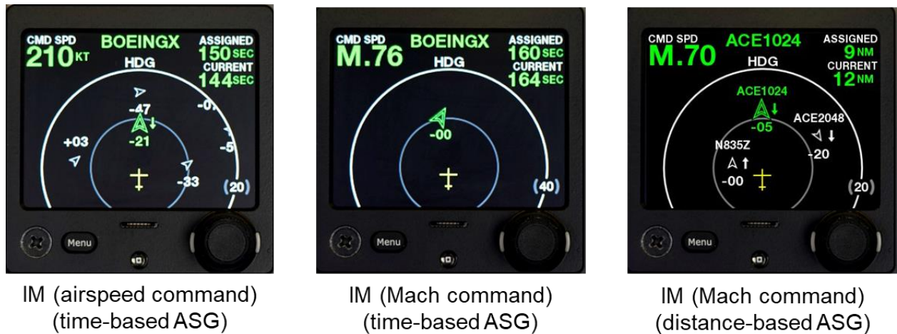
Figure 3 – AGD display for various operating modes of the ACSS I-IM implementation Copyright ACSS. Used by permission.
