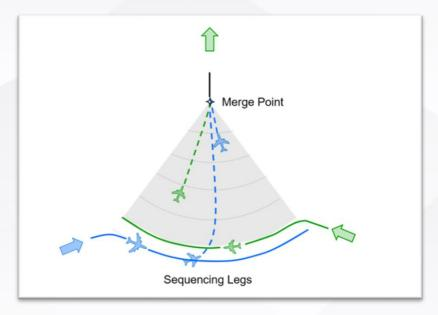
PMS consists of a merge point and two or more sequencing legs equidistant (vertically separated) from the merge point.
