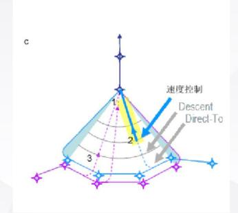
For PMS operation, there is usually only one "direct to" instruction, and the separation is established by the timing of instruction.
