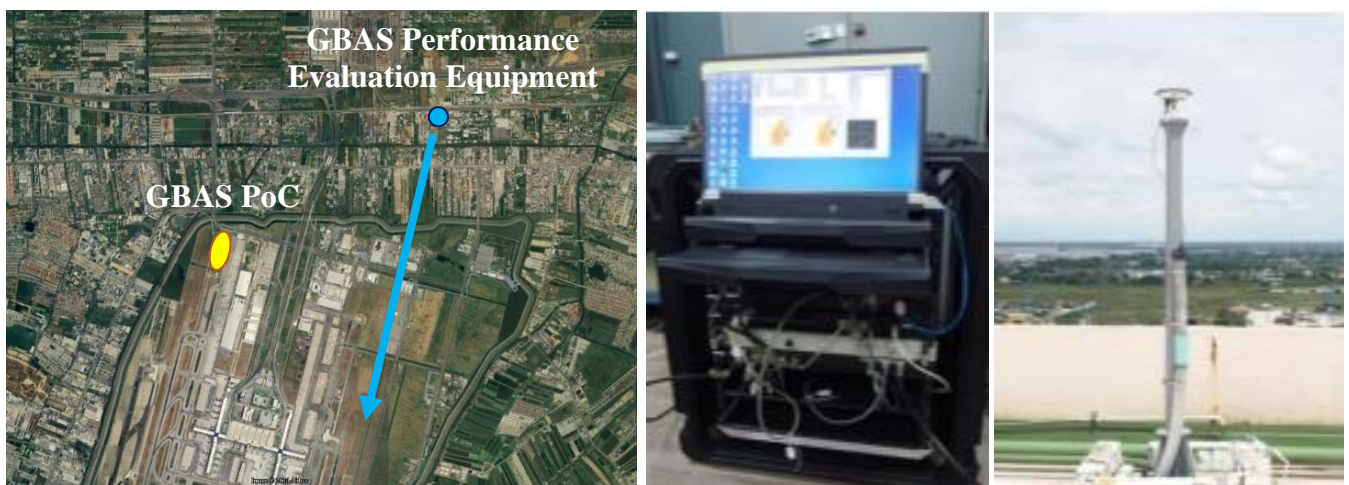
Figure 12. Location of GBAS Performance Evaluation Equipment and GBAS PoC (Left), GBAS Performance Evaluation Equipment (Middle), GNSS Antenna for Performance Evaluation (Right)
