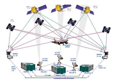
The GPS information collected by these 15 reference stations is forwarded to the INMCC either by terrestrial or satellite communication network. At INMCC, GPS information is <u>processed</u>, and correction (augmentation) messages are generated.
