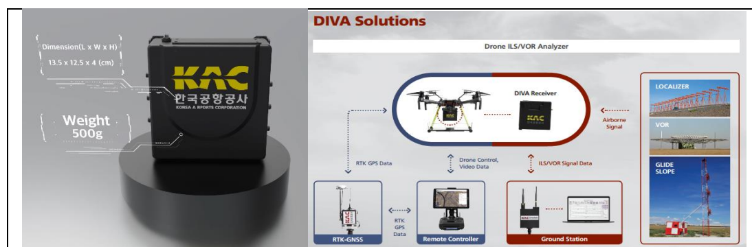
Figure 1. Drone system configuration diagram for navigational Aids check and software for analysis
