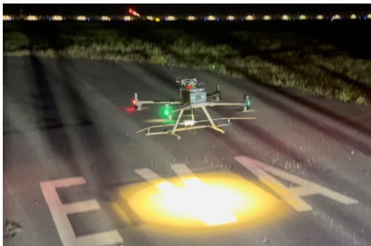
Fig. 1 – The four-rotor drone equipped with specially designed signal receiver for flight inspection trial
