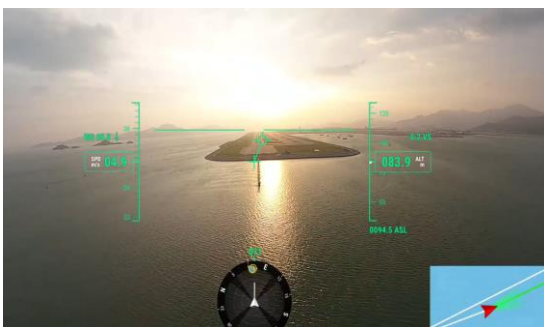
Fig. 3 – Drone performing low approach profile to inspect the ILS signal
