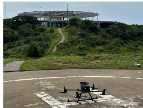
Fig. 2 – Drone to perform orbiting to measure DVOR bearing error
