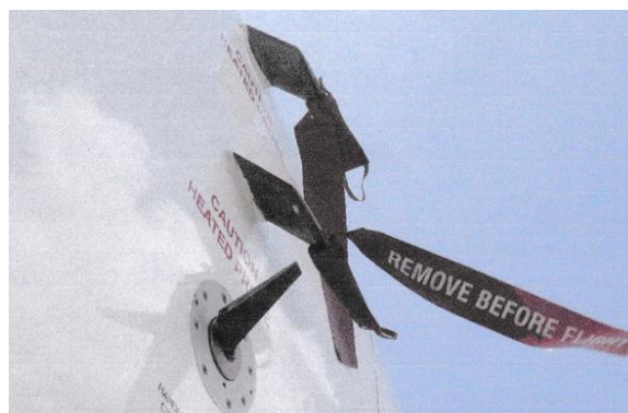
Figure 4: Pitot probe covered to avoid insects from entering the probe ( Source: FRIM Report, 2022 )
