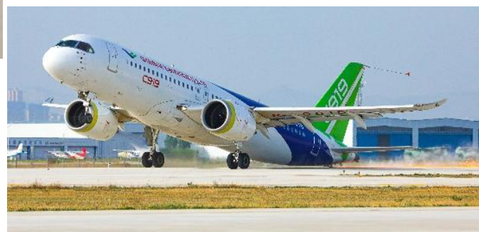
Minimum Unstick Speed Test. Shannxi Yanliang
