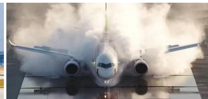
Minimum Unstick Speed Test. Shannxi Yanliang
