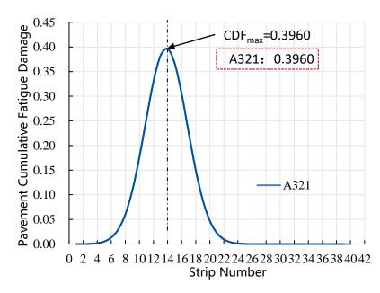
Step 8: As the A321 is the aircraft type with the maximum ACR in the combination,  $PCR = max(PCR_1, PCR_2, PCR_3) = 518.24$ , rounded to 520
