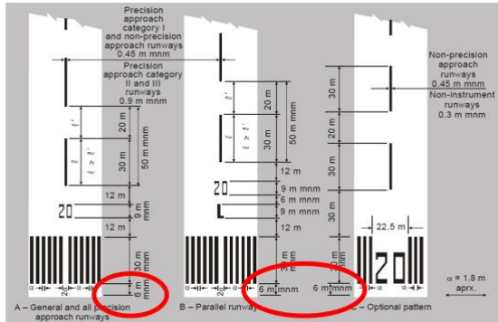
Figure 5-2. Runway designation, centre line and threshold markings
