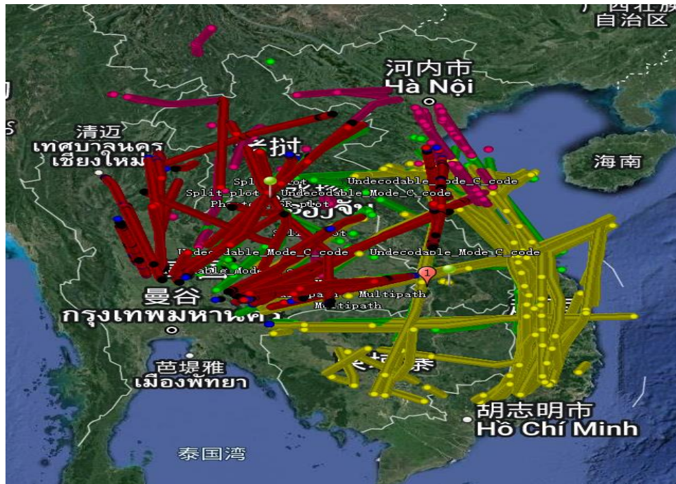
Figure 7 Actual Target Tracking Radar and ADS-B Coverage in LAOS
