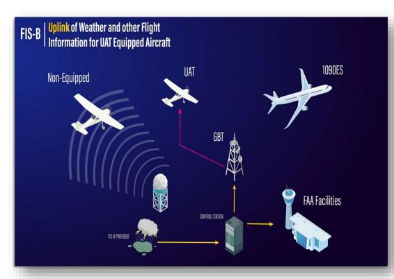
The yellow arrows show ground-based data flow from the Flight Planning systems to the control station, then the ground-based towers (GBT). The pink arrows show the transmitted data flow to UAT equipped aircraft.
