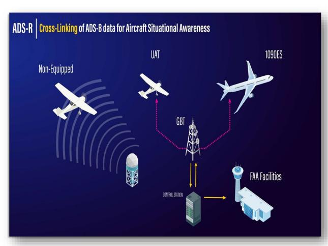
The yellow arrows show ground-based data flow from the receiver about non-ADS-B equipped aircraft to the control station, then the ground-based towers (GBT). The pink arrows show the transmitted data flow to ADS-B equipped aircraft.
