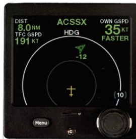
ADS-B In Guidance Display (AGD)
