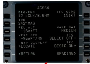
Multi-Purpose Control Display Unit (MCDU)
