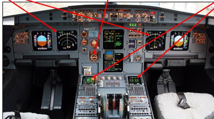
Figure 1 – ACSS avionics being installed in AAL A321s (the only new hardware is the AGD) Copyright ACSS. Used by permission.
