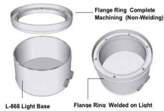
L-868 Light Base Flange Ring Welded on Light
