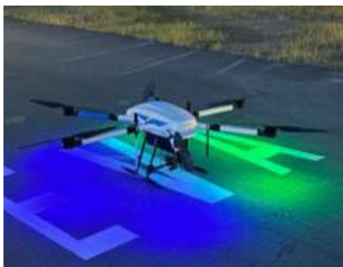
Fig. 1 – The six-rotor drone for inspecting LOC signals
