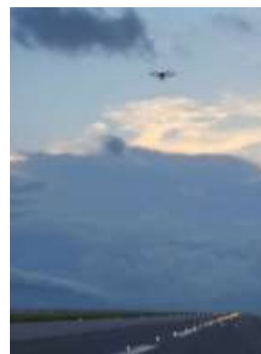
Fig. 2 – Drone flying along the center line over the North Runway to inspect LOC signals
