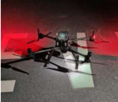
Fig. 3 – The four-rotor drone for inspecting PAPI lights
