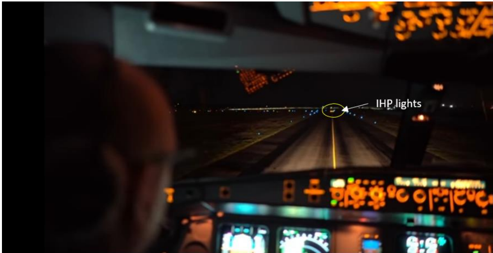
Figure 4. IHP lights form distance on a taxiway with taxiway edge lights
