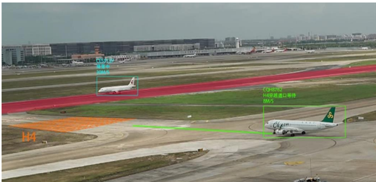
Figure 5 Hold line video detection
