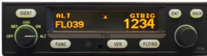
Figure 3.4 TT31 Mode S Transponder from TRIG
