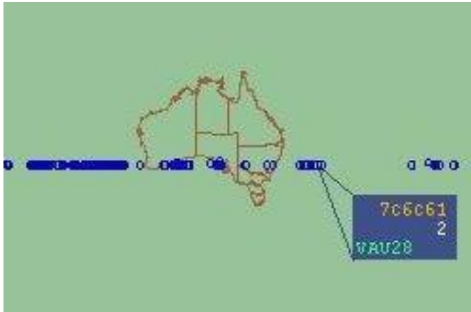
Figure 1 - Track Jumping problem with TPR901
