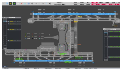
Figure 2 Tower controller ground system
