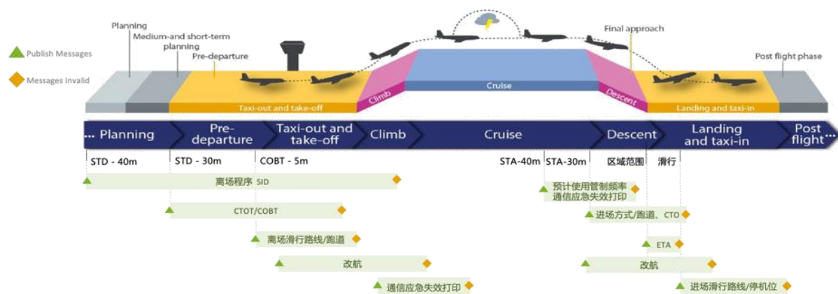
Figure 1 Verification scheme of Data-link Air Traffic Control Services for All Flight Phases
