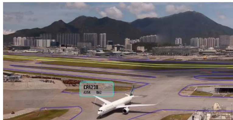
Detection and labelling of an aircraft on taxiway
