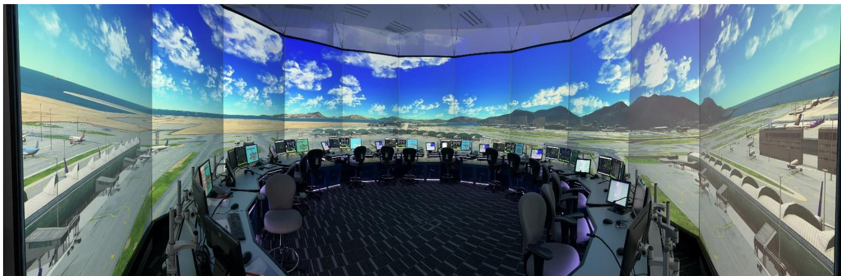
New 360° CTS showing simulated aerodrome environment at ATC tower
